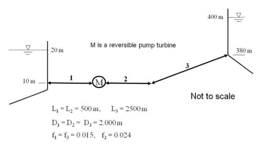
Assume efficiency of machine – acting either as a pump or a turbine – is 90%; assume the design velocity is 3.00 m/s
