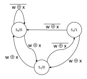
Using the state codes below, derive the next-state logic functions and the output logic function. Use  $Y_1$  and  $Y_0$  as the signal names for the next-state logic; use z as the output signal name. Use Karnaugh maps to minimize your logic functions, taking advantage of don't-cares if possible. Show your work; you can also use the next page.
