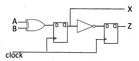
Write Verilog code for the logic circuit:
