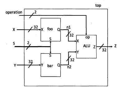
[5 marks] Write structural Verilog for the circuit top, assuming that the modules foo, bar, and ALU are already specified, with the following port orderings: foo (X, S, Q), bar (Y, S, Q), ALU (X, Y, op, Z). Use the signal and port names shown in the figure.
